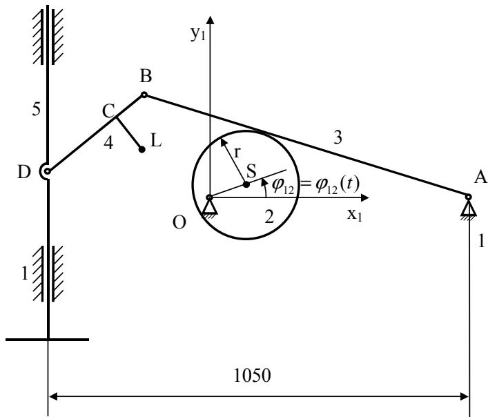
D:  $\overline{OS} = 100 \text{ mm}$ ,  $r = 130 \text{ mm}$ ,  $\overline{OA} = 650 \text{ mm}$ ,  $\overline{AB} = 850 \text{ mm}$ ,  $\overline{BD} = 300 \text{ mm}$ ,
